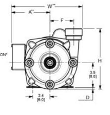
Maximum Solids Handling Capacity: 1/8" Diameter
